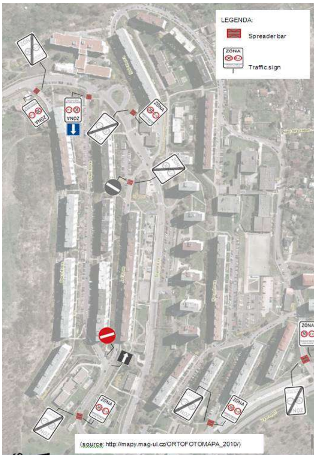
Figure 3– Schema of the modification into a TEMPO 30 zone (sample area Doběčice)
