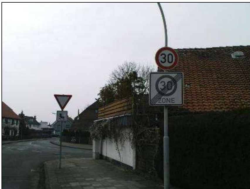
Figure 2.22 - Confusing road signs for TEMPO 30 zone (Germany)
